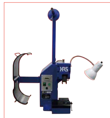
Automatic crimping press (Type CM-105C)
