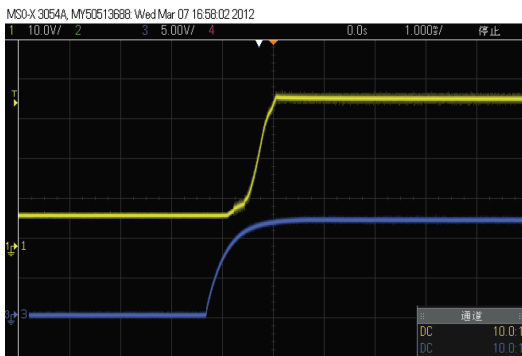
Start up Waveform (CH1=V OUT(AC) , CH2=V IN(AC) )
