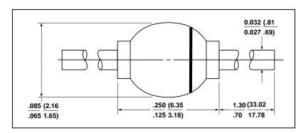
FIG. 106: Axial Lead Rectifier Outlines
