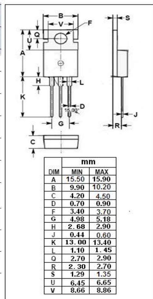
**isc N-Channel MOSFET Transistor****IPP039N04L, IIPP039N04L****ELECTRICAL CHARACTERISTICS** $T_c=25^\circ\text{C}$  unless otherwise specified
