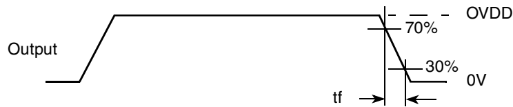
Figure 7. Definition of Timing for Standard- and Fast-Mode
