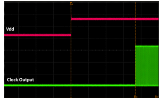
Figure 16. Startup Waveform vs. Vdd
