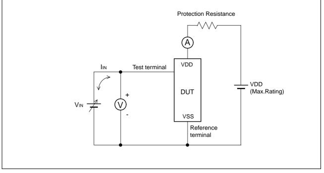
Note : The voltage V<sub>IN</sub> is increased gradually and the current IIN of 300 mA at maximum shall flow. Confirm the latch up does not occur under  $I_{IN} = \pm 300$  mA. In case the specific requirement is specified for I/O and  $I_{IN}$  cannot be 300 mA, the voltage shall be increased to the level that meets the specific requirement. • C-V method of Latch-Up Resistance Test
