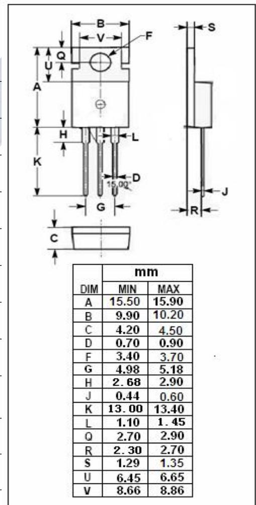
**isc N-Channel MOSFET Transistor**
