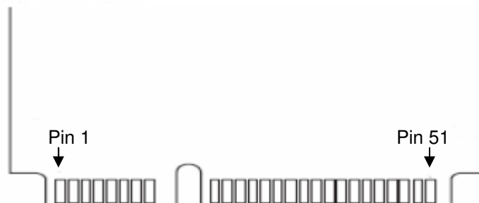
Figure 1-2 Apacer mSATA M4 pin assignment
