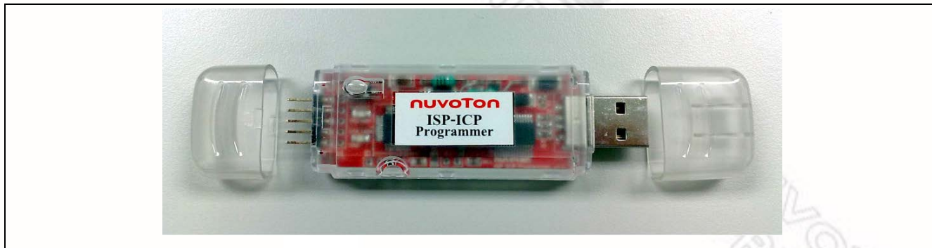
Figure 27–2 Nuvoton ISP-ICP Programmer
