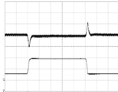
Output voltage response to load current step-change (6.25-18.75-6.25 A) at: T_{P1} = +25^\circ\text{C} , V_i = 53\text{ V} . Top trace: output voltage (200 mV/div.). Bottom trace: load current (10 A/div.). Time scale: (0.1 ms/div.).
