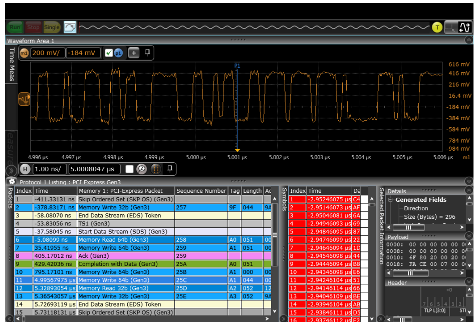
Z-Series decoding the PCI Express Gen 3 packets.
