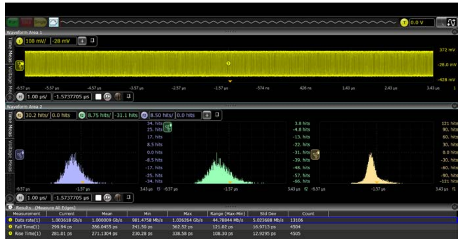
With its flat frequency response and low noise, the Z-Series is able to accurately measure jitter components such as ISI.
