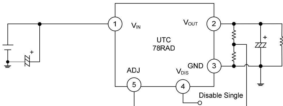
\* C<sub>I</sub> is required if regulator is located an appreciable distance from power supply filter. [C<sub>I</sub> > 0.33μF (Electrolytic)]
