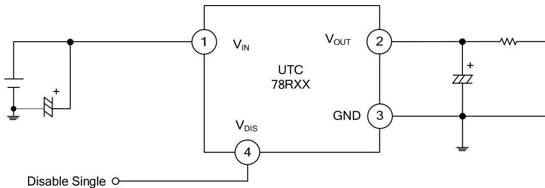
\* C<sub>I</sub> is required if regulator is located an appreciable distance from power supply filter. [C<sub>I</sub> > 0.33μF (Electrolytic)]
