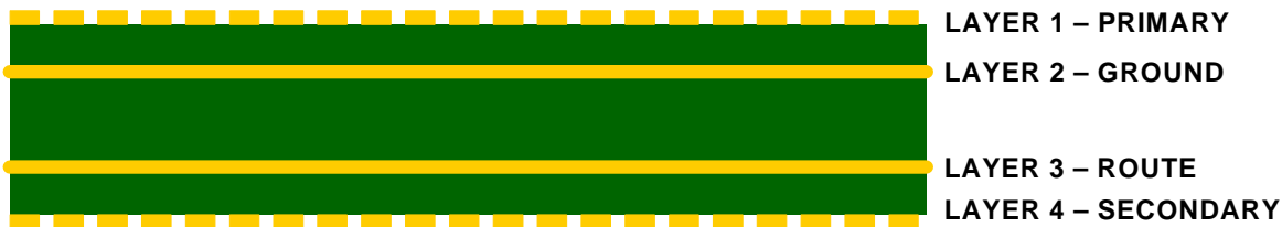
Figure 7. Four Layer Stackup
