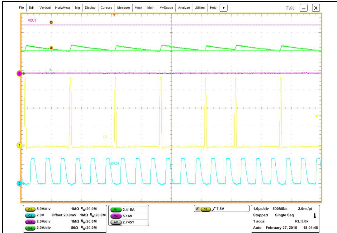
Figure 23. Valley current sense operation in overcurrent condition
