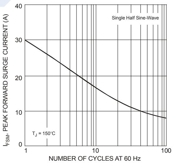
Fig. 4 Max Non-Repetitive Peak Forward Surge Current
