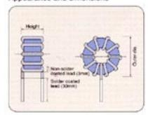
Inductance tolerance: ±25%, Winding wire type:1UEW Note Standard number of turns could vary with inductance. The above figures are for reference only.
