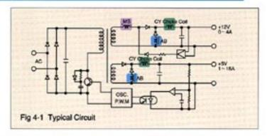
Cauties: Iron amorphous alloy has comparatively high magnetostriction, and ringing may be generated at audio frequency
