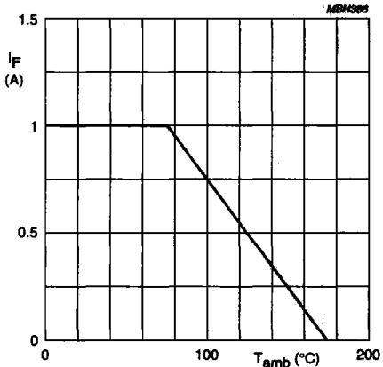
Fig.2 Maximum forward current as a function of ambient temperature.
