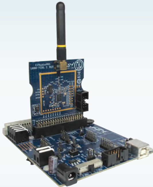
Si1000 TARGET BOARD WITH EZRadio® TEST CARD
