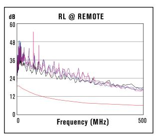
Note: Above graphs illustrate the main ethernet test results of the CarlisleIT Octax<sup>™</sup> connectors and cable 26463/1A042X-8(LD). These charts were produced by using Fluke DTX 1800 test equipment with TIA/EIA-568 CAT 6A specification, 180 ft of cable, and 4 connectors. Drawings, test report, and other contact arrangements will be available upon request. Contacts are included with connector.
