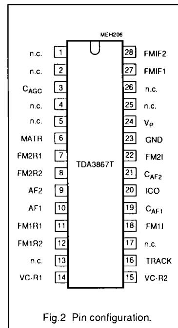
Fig.2 Pin configuration.
