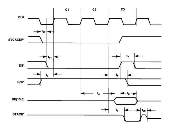
Figure 6-10. Synchronous Service Acknowledge Cycle Timing
