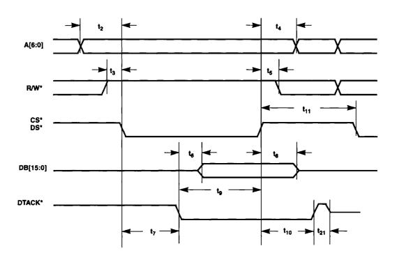
Figure 6-3. Asynchronous Read Cycle Timing
