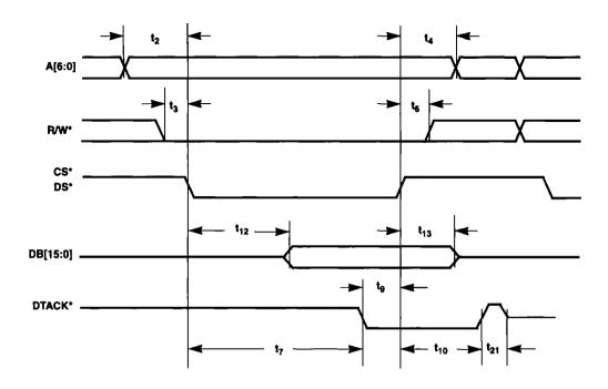
Figure 6-4. Asynchronous Write Cycle Timing
