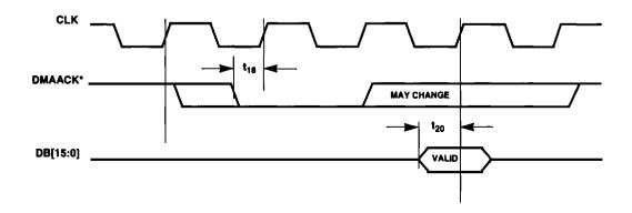
Figure 6-7. Asynchronous DMA Write Cycle Timing
