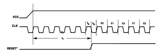
Figure 6-1. Reset Timing
