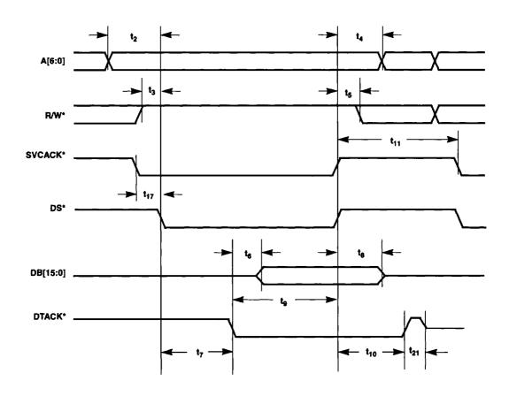
Figure 6-5. Asynchronous Service Acknowledge Cycle Timing
