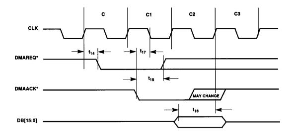
Figure 6-11. Synchronous DMA Write Cycle Timing
