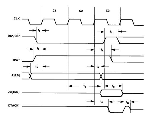
Figure 6-8. Synchronous Read Cycle Timing
