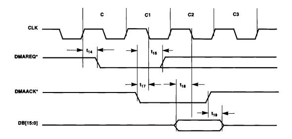
Figure 6-12. Synchronous DMA Read Cycle Timing
