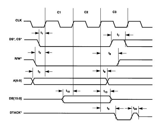
Figure 6-9. Synchronous Write Cycle Timing
