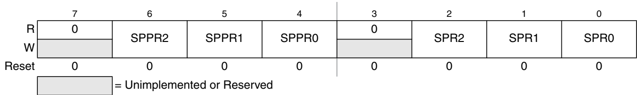
Figure 21-5. SPI Baud Rate Register (SPIBR)
