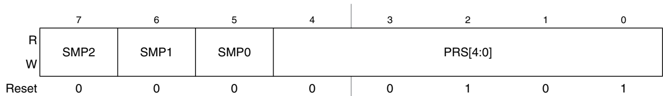
Figure 13-7. ATD Control Register 4 (ATDCTL4)
