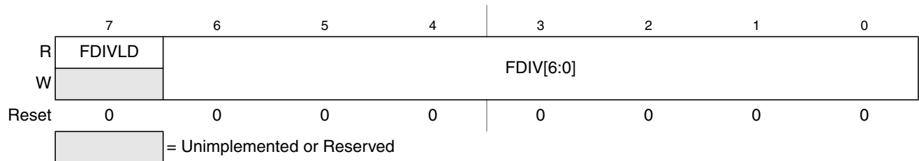
Figure 26-5. Flash Clock Divider Register (FCLKDIV)
