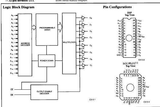
For LCC/PLCC only: Pins 1 and 17 are common and tied to the die attach pad. They should not be used.
