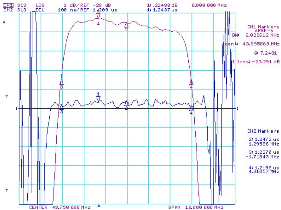
Figure-2 S21 Response(Pass Band/Span=10MHz)
