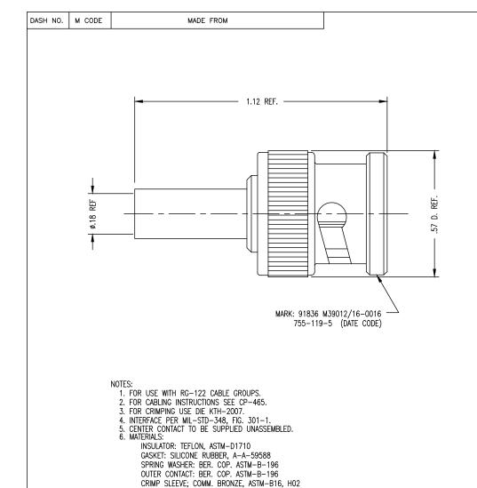
ALL OTHER METAL PARTS: BRASS, ASTM-B16 7. FINISHES: CENTER CONTACT: GOLD PLATE PER ASTM-B488 ALL OTHER METAL PARTS: SILVER PLATE PER ASTM-B700
