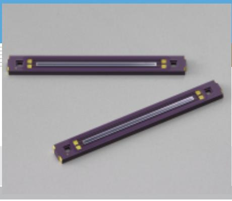
S8543 is a one-dimensional PSD with a long, narrow active area sealed in a surface mountable chip carrier package. The active area of 0.7 × 24 mm delivers excellent position detection characteristics.
