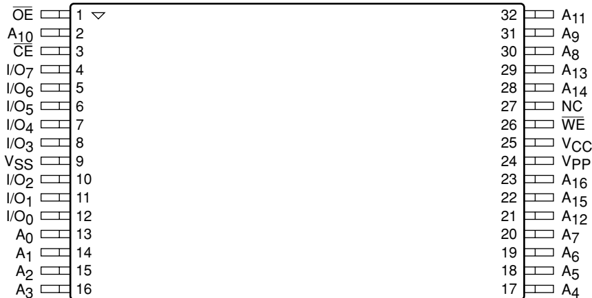
TSOP Package (Reverse Pinout) (TR, HR)
