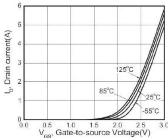
Figure 2. Transfer Characteristics
