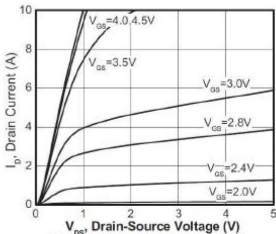
Figure 1. Output Characteristics
