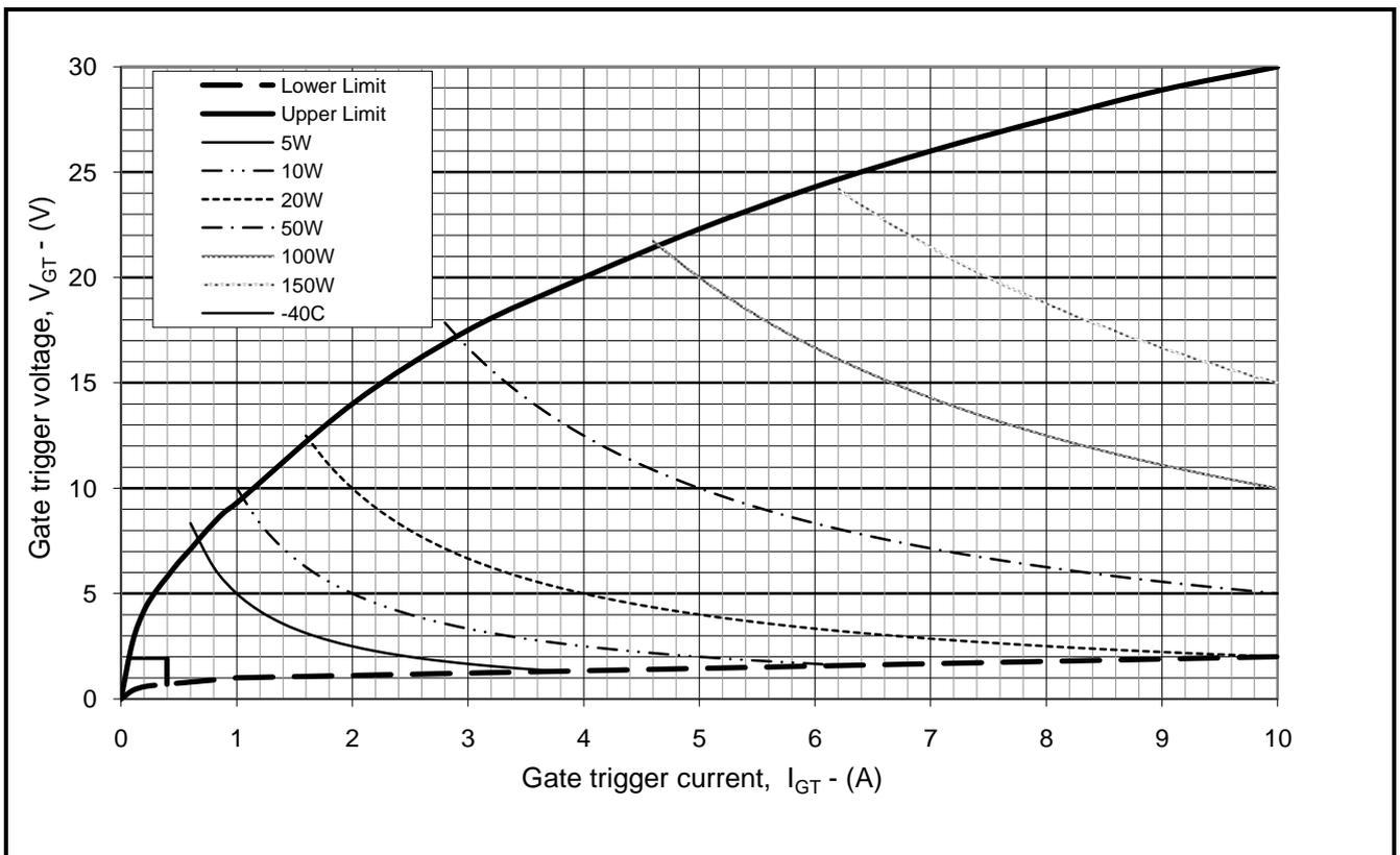
Fig. 15 Gate characteristics
