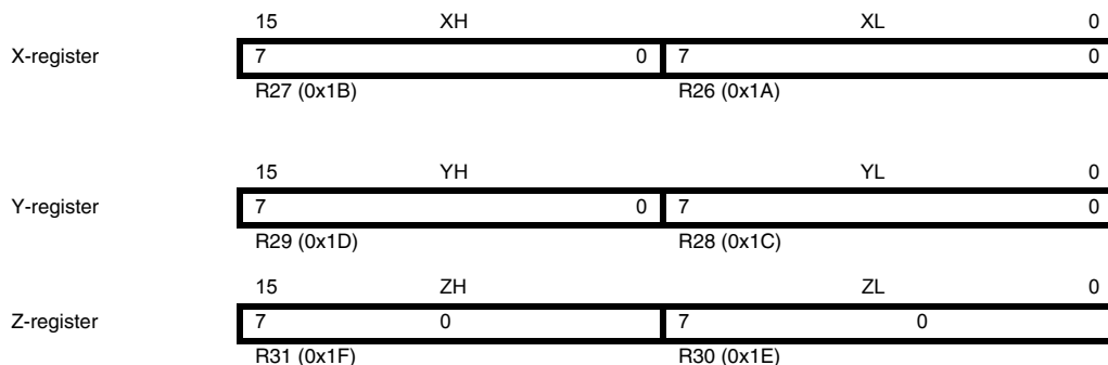
Figure 7-3. The X-, Y-, and Z-registers.
