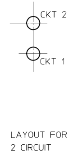
RECOMMENDED PCB HOLE LAYOUT COMPONENT SIDE
