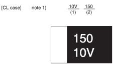
note 2) voltage code and capacitance code are variable with parts number
