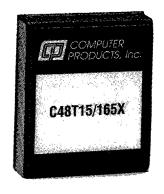
The C series consists of a family of triple output DC/DC converters that provide 10 watts of isolated, well regulated output power. Models are available with outputs of either ±12V or ±15V at 165 mA and 5V at 750 mA. The units offer better than 500VDC isolation and line and load regulation better than 1.0%. All models are encapsulated in 3.0 x 2.56 x 0.75 inches metal cases designed for optimum noise containment. EMI/RFI protection is provided by a six-sided continuous package shield
