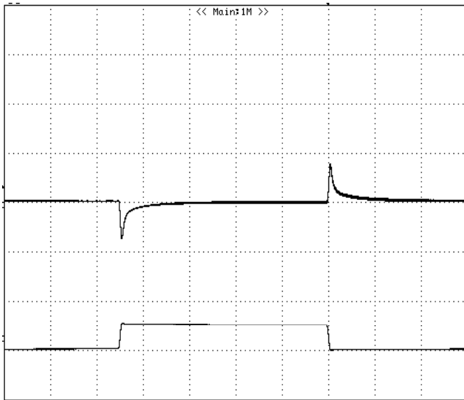
Figure 8: Output voltage response to step-change in load current (75%-50%-75% of I_o , max; di/dt = 0.1A/\mu s ). Load cap: 10\mu F , tantalum capacitor and 1\mu F ceramic capacitor. Top Trace: V_{out} (100mV/div, 500us/div), Bottom Trace: I_{out} (5A/div). Scope measurement should be made using a BNC cable (length shorter than 20 inches). Position the load between 51 mm to 76 mm (2 inches to 3 inches) from the module..
