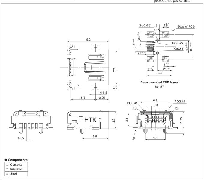
Mating connectors: USB mini-B series connector for cable (USB 2.0 standard)
