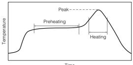
Recommended soldering conditions for flow
