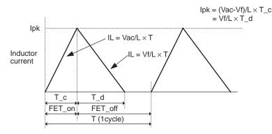
Given that the period when current flows into coil is
