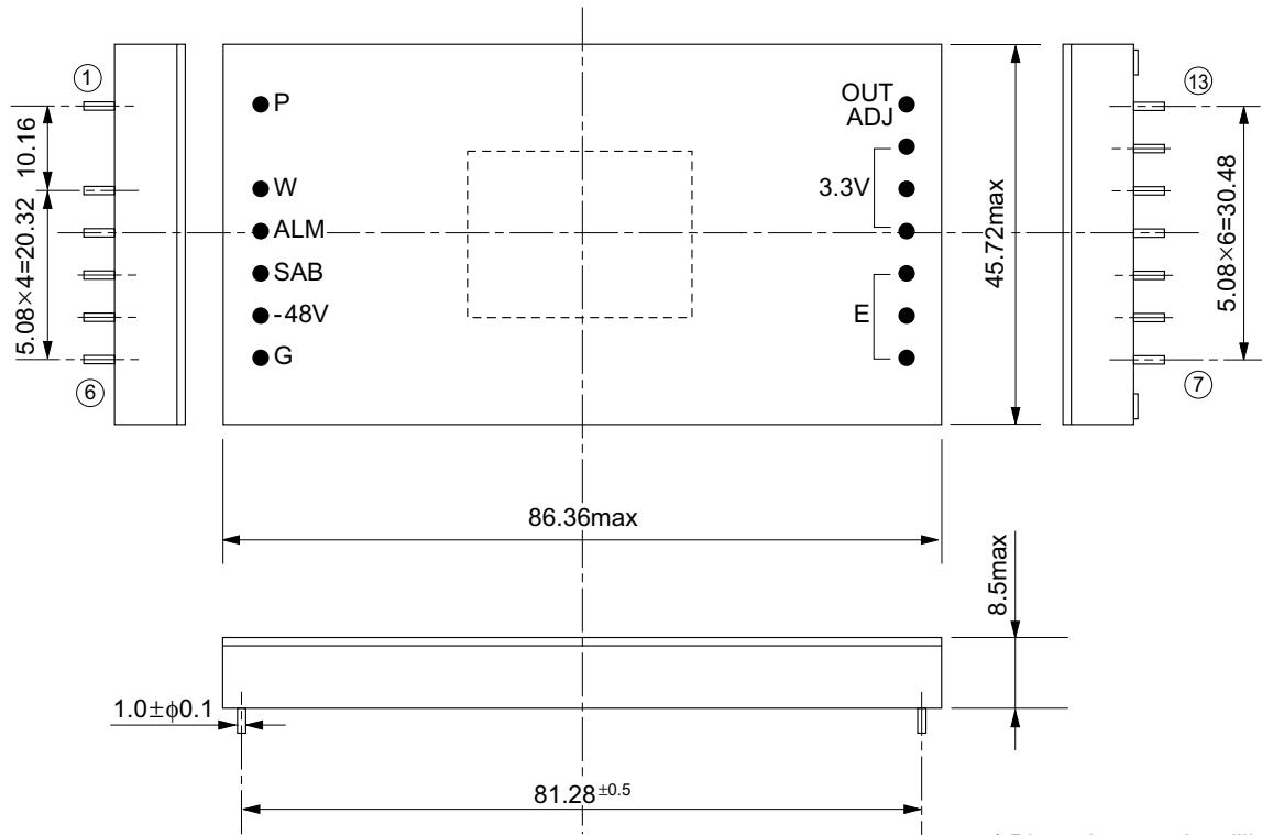
\* Dimensions are in millimeters.
