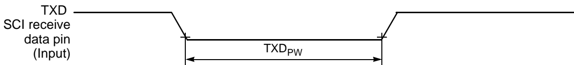
Figure 10-17 TXD Pulse Width
