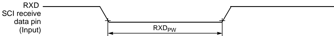
Figure 10-16 RXD Pulse Width
