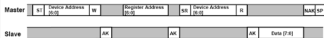
Figure 7. Single Byte Read - The Master is reading one address from the MMA7450L
