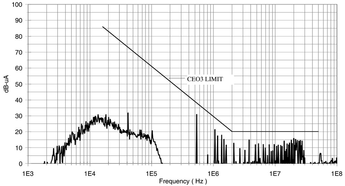
**Figure 3. Conducted Emissions, Return Lead**
