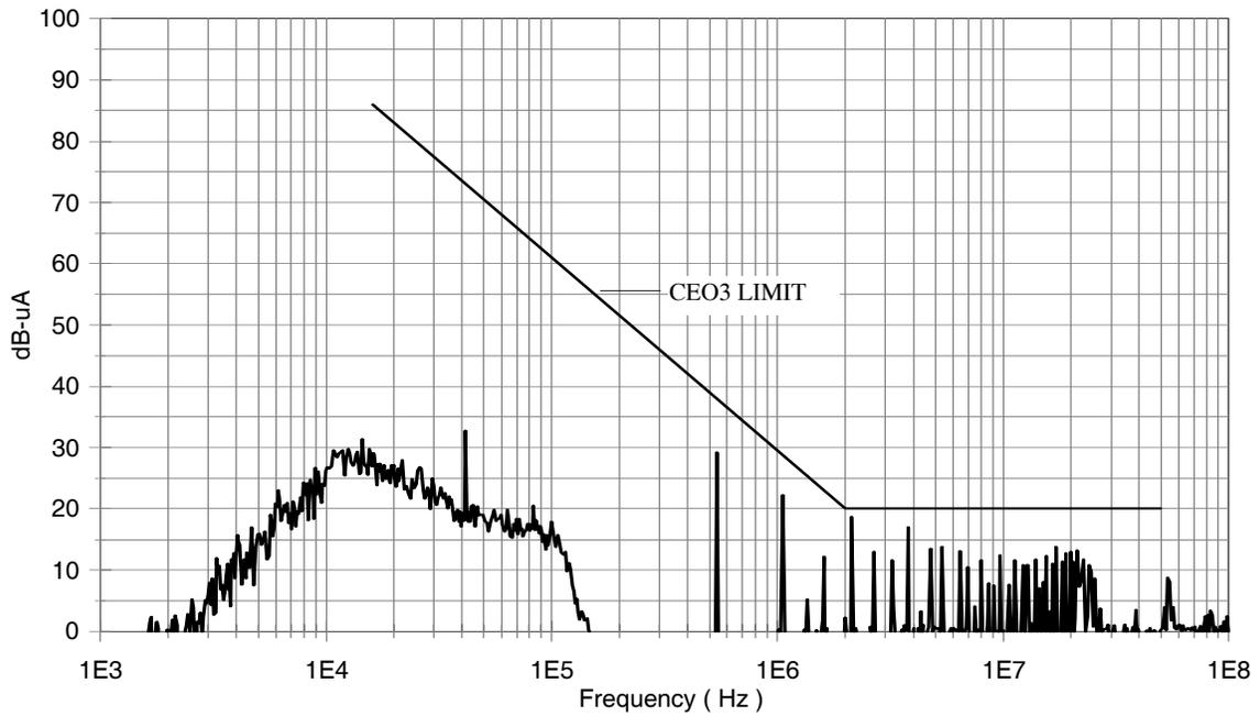
Figure 4. Conducted Emissions, Common Mode
