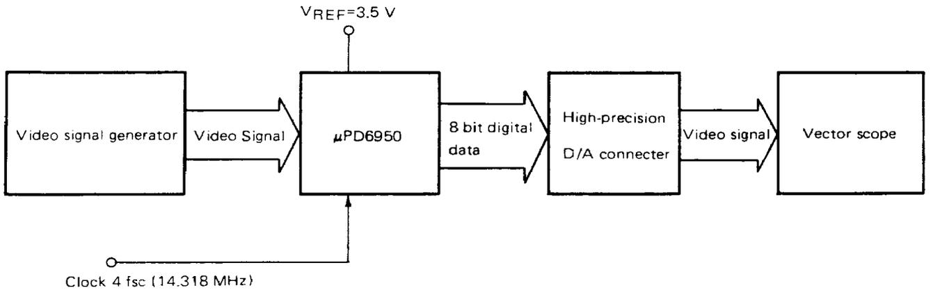
The video signal from the video signal generator is 40 IRE Ramp signal.
