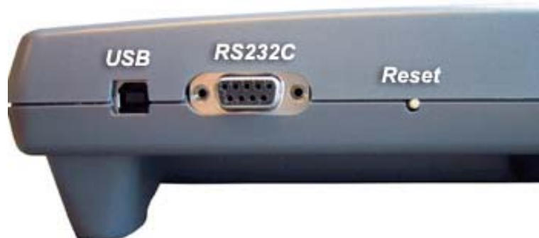
Figure 3-6. USB-, RS-232C-communication, and Reset Button
