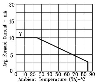
Fig5. MAX AVERAGE FORWARD CURRENT VS. AMBIENT TEMPERATURE.
