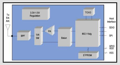
The W2SW0001 SiP delivers a complete, WLAN radio solution. All functionality, including the radio modem, interface control, diagnostics, timing, and power regulation are included in a certified compact ready to integrate package.
