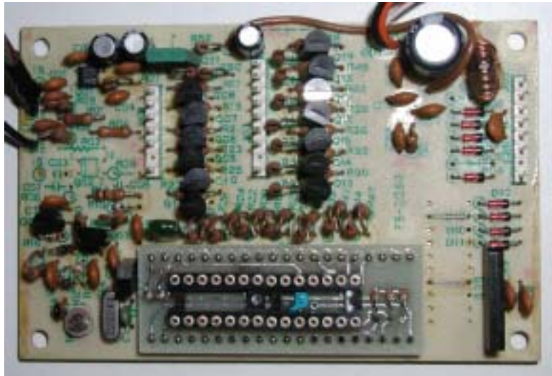
Fig. 8 Completed COUNTER DISPLAY UNIT (w/o PIC16F873)
