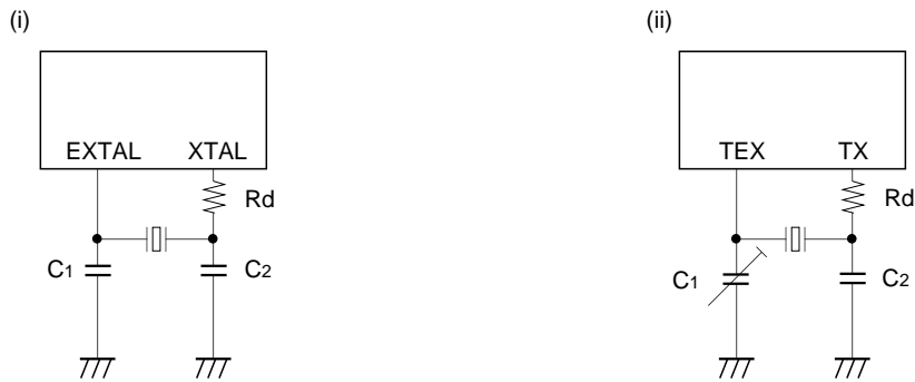
Fig. 12. Recommended oscillation circuit
