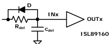
FIGURE 18. SETTING DELAYS WITH A RCD NETWORK
