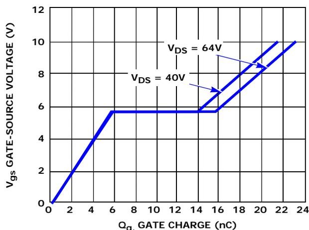
FIGURE 19. MOSFET GATE CHARGE vs GATE VOLTAGE
