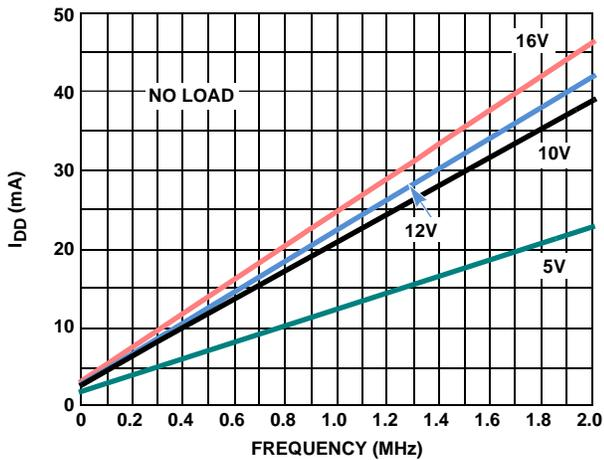
FIGURE 11. I<sub>DD</sub> vs FREQUENCY (+25°C)
