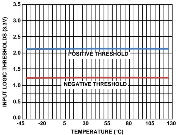
FIGURE 13. INPUT THRESHOLDS
