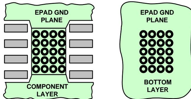
FIGURE 20. TYPICAL PCB PATTERN FOR THERMAL VIAS
