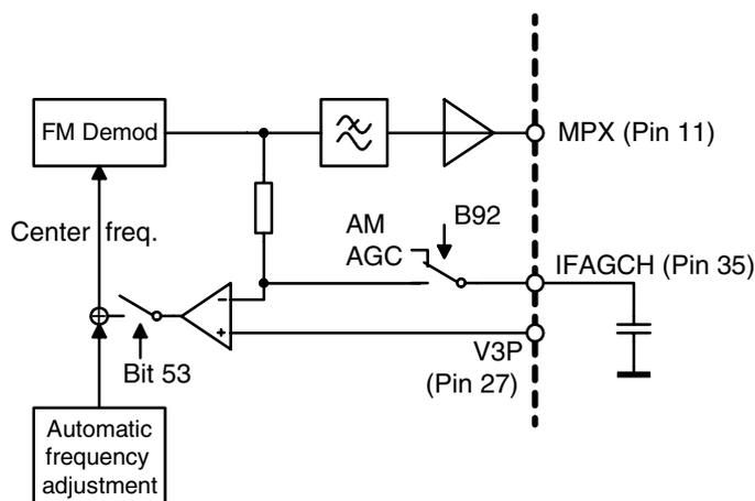
The center frequency of the FM demodulator can be adjusted by means of bit 56 to 59. At the center frequency, the DC voltage at the MPX output pin 11 is equal to the MPX offset voltage that can be measured at pin 11 while MPX mute is active (bit 7 = 1). This adjustment will affect the center frequency of all integrated filters as mentioned before.
